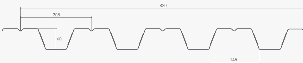
Image 1 – Geometry of H60 profile
