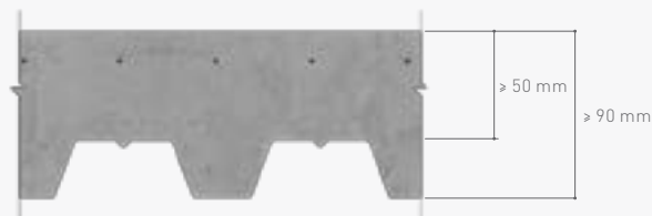
Image 5 – Cross section of the slab
